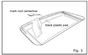
6) Mark the roof centerline on the flange using the black plastic pad on the headliner for reference. (Fig. 3)
