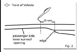
5) Measure 23mm forward from the edge shown in Fig. 2 and mark the location on the flange. Repeat for driver side.
